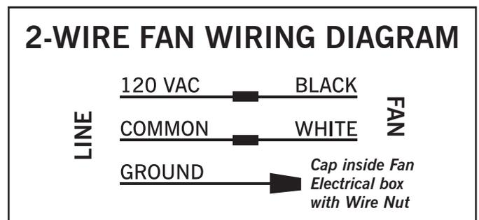
Note: Some of our fan models use motors that do not utilize a ground wire. This wire configuration is safe and allowable under our ETL safety listing. If the fan being installed was constructed with the 2-wire configuration (no ground), the ground wire from the Line supply should be capped with a wire nut inside the electrical box at the fan.
