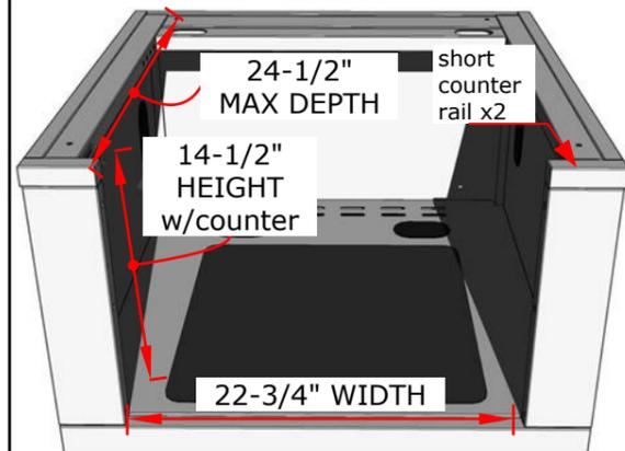
Removing the two center panels allows Kamado to Bulge out of front opening at 22-3/4"W with an internal 24-1/4"W x 23-1/2"D x 14-1/2"H w/3/4" Counter
