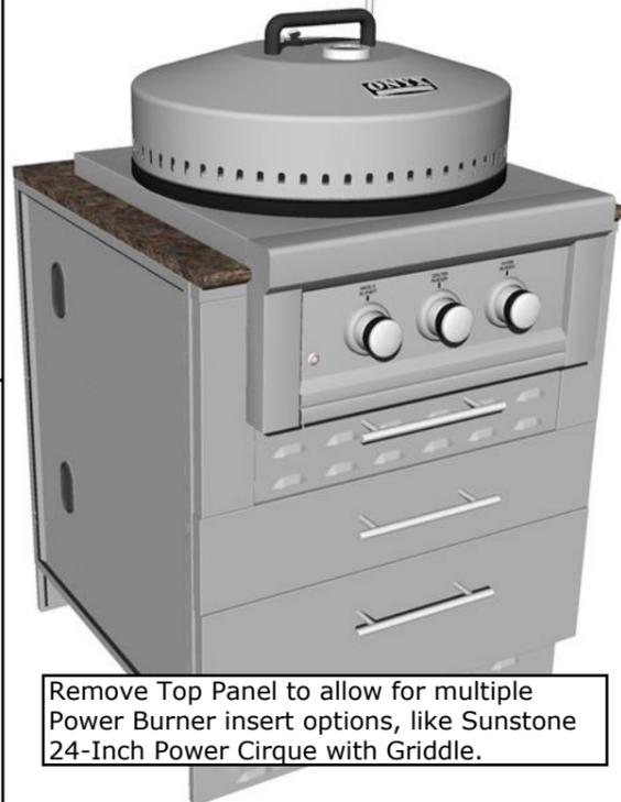
Removing top panel allows a product insert dimension of 22-3/4" Width x 8-1/2" Height x Max 24-1/2" Depth. Add 1 Inch Height Counter to provide a Cut-Out height of 9-1/2"
