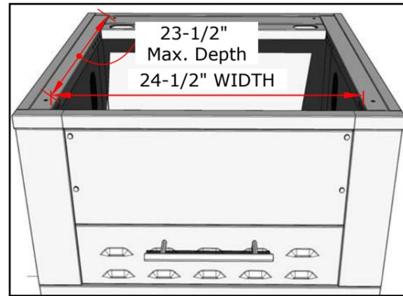
With full panel installed, this provides a maximum insert dimension of 24-1/2"W x 23-1/2"D x 14-1/2"H w/3/4" Counter
