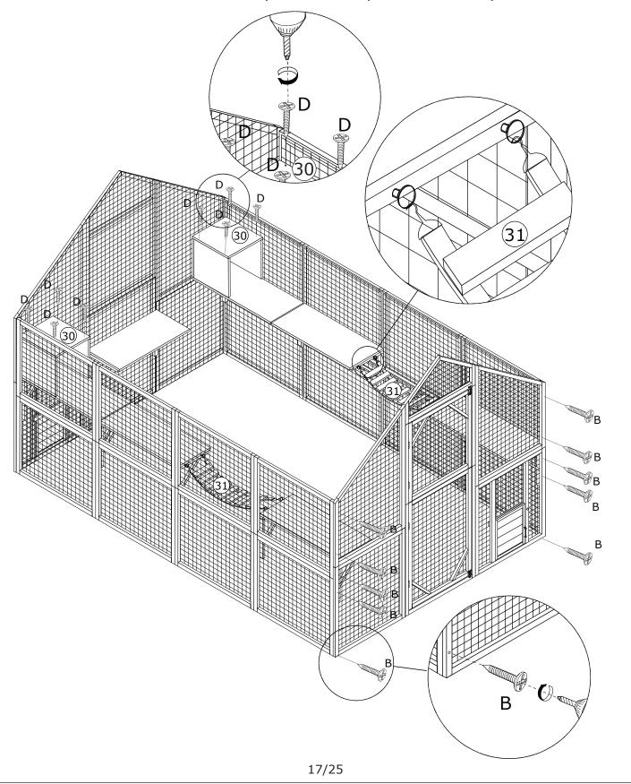
A x 26 When turning the screws, please do it slowly and keep the direction vertical. M3.5 x 50 mm 16 19 18 (17)18
