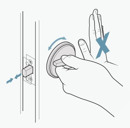
With the door closed in its normal position, does the latch engage properly and hold the door in the closed position? Does the bolt lock and unlock without any friction?
