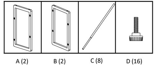
Connect large ends of EXPANDABLE RODS (C) to RIGHT SIDE FRAME (B) with THUMB SCREWS (D) through frame holes and screw into EXPANDABLE RODS (C). Connect small ends of EXPANDABLE RODS (C) to LEFT SIDE FRAME (A) with THUMB SCREWS (D).
