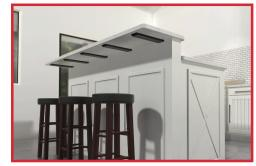
**6.** Check once again that the counter top is level. Once level, caulk around the brackets with clear silicone to hold your counter top securely.
