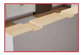
2. Rout or chisel a 2.5" wide by 0.5" deep pocket on top of the knee/pony wall. This "pocket" will allow the bracket to sit flush with the top of the wall. (Make sure it is flush)
