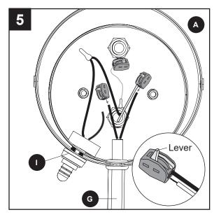
Remove the hex nut preassembled to plug button (EE). Then insert the plug button (EE) through grommet (I) and secure with the hex nut.
