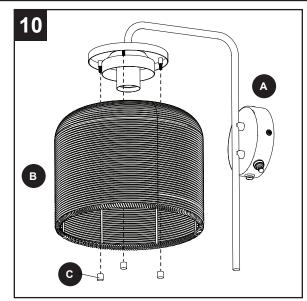
To prevent water, rain, or moisture from entering fixture (A), use waterproof caulk (sold separately) to seal the perimeter.
