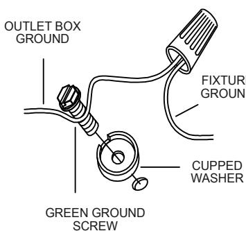
Connect wires according to the chart below
