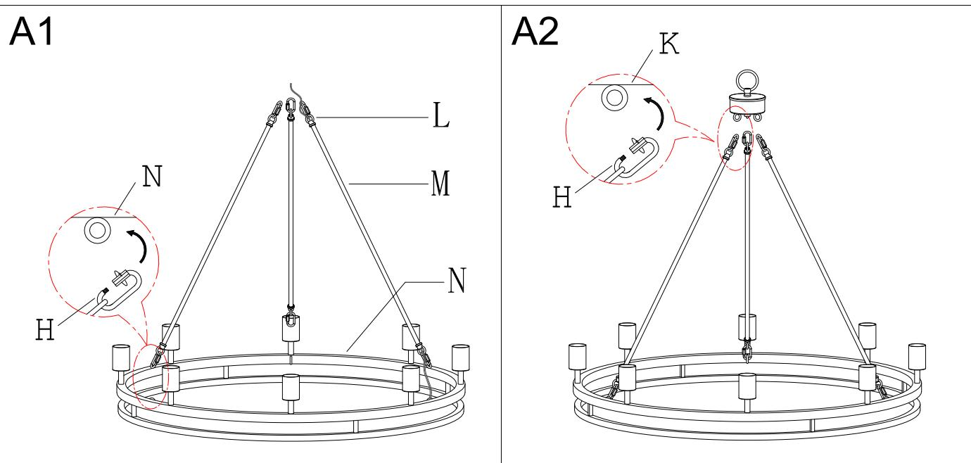
**Step A1 »** Open the quick link (H) on one end of the rod (M) as shown in the figure, pass the quick link (H) through the ring on the iron frame (N), and then close the quick link (H).
