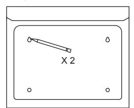
For brick or other masonry wall, insert a plastic anchor (included) into each hole. Tap in gently if necessary. This step is not required if mounting on a wood wall.
