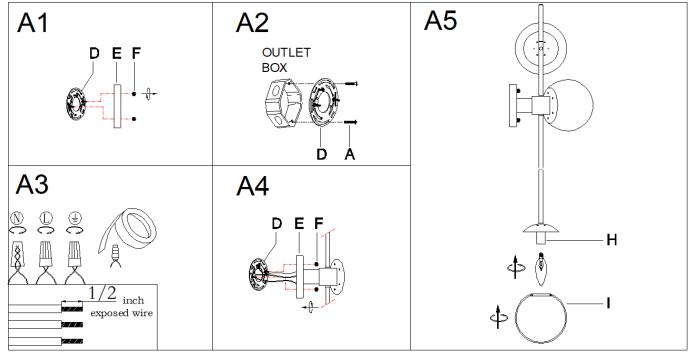
Step A1: Unscrew the ball knob(F) from the back plate(E) then gently remove the mounting plate (D). Step A2: Secure mounting plate (D) to outlet box with mounting screws (A).
