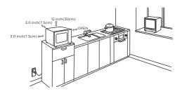
A minimum clearance of 3.0 inches (7.5cm) is required between the oven and any adjacent walls. One side must be open.
