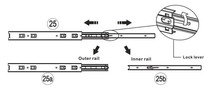
Soft Reminder: Before installing the drawer slides, you need to disassembly it into two parts. The outer guide 25A is installed on the inside of the cabinet; the inner guide 25B is installed on the outside of the drawer;
