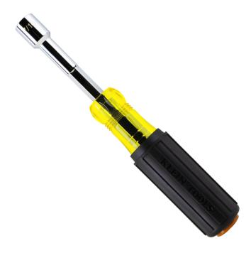
Klein's Color-Coded Hollow-Shaft Heavy-Duty Nut Driver features a fully pass through driver for driving nuts on threaded rod and prevents bottoming out. Cold forged steel wrench assist provides greater torque, especially helpful for breaking stubborn nuts and bolts free. The handle is color-coded and dome-stamped to easily identify the common 7/16-Inch hex size needed for the job.
