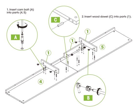
3. Attach part (1) to the wood dowels of parts (4) and (5) using cam lock (B) and Phillips head screwdriver.
