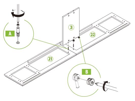
2. Attach part (3) to parts (21, 22) using cam lock (B) and Phillips head screwdriver.
