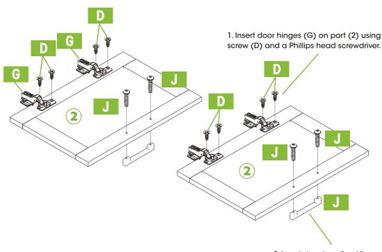
2. Insert door handles (J) on part (2) using screw (J) and a Phillips head screwdriver.
