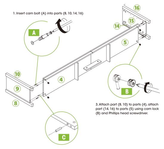
2. Insert wood dowel (C) into parts (4,5).
