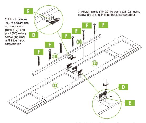
1. Attach pieces (E) to secure the connection in parts (21) and part (22) using screw (D) and a Phillips head screwdriver.
