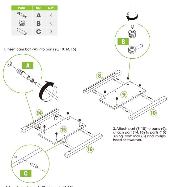
2. Insert wood dowel (C) into parts (9, 15).
