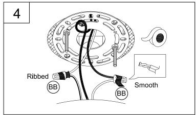
4. Strip 3/8" of insulation from the electrical wire ends. Using wire connectors (BB), connect RIBBED fixture wire to the WHITE supply wire from the outlet box; connect the SMOOTH fixture wire to the BLACK supply wire from the outlet box.
