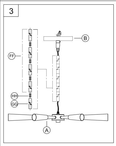
NOTE: During this step, determine the hanging length of your fixture by adding or removing pipes. The electrical and ground wire may also optionally be cut to length.
