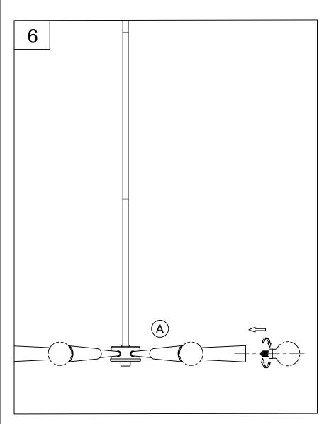
6. Thread the lamps (not included) into the fixture sockets. Use 60-watt MAX incandescent candelabra base lamp, SBCFL or SBLED.
