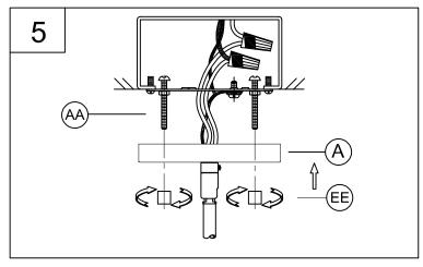
5. Pass the screws through the two holes in the canopy. Secure the fixture (A) to the screws (AA) using the two cylinder nuts (EE). Tighten securely.
