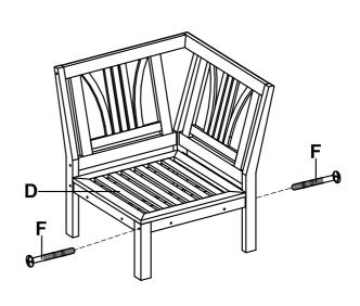
Next, attach the seat (D) into pre-assembled of side frames and secure using 2 1/4" bolts (F).
