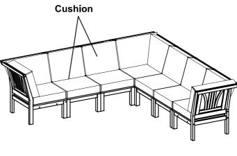
Joint all the corner chairs and other chairs as shown. Secure using 2" bolts from underneath of seat. Make sure all parts are correctly connected and tighten all bolts using screwdriver.
