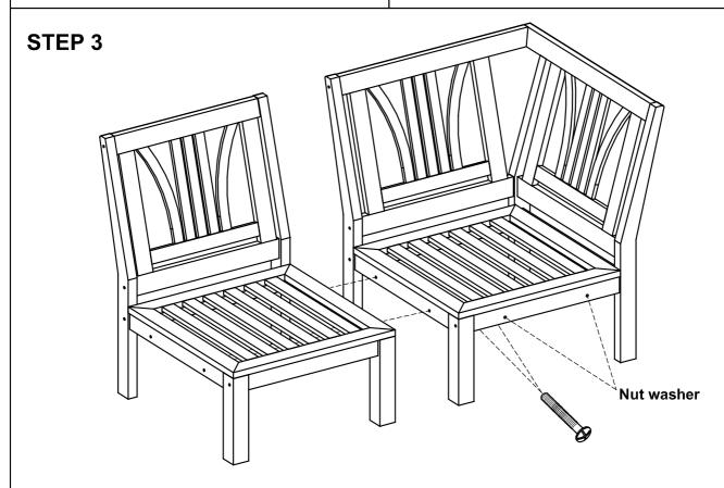
Next, joint the corner chair with other chair and secure using 2" bolts (G) from underneath of seat.
