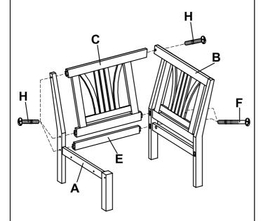
Attach side frame (A) and back support (C) into side frame with support (B) and apron (E).
