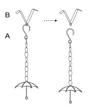
**STEP 2** Slide the Gutter Clip (B) into the rain gutter drain hole.
