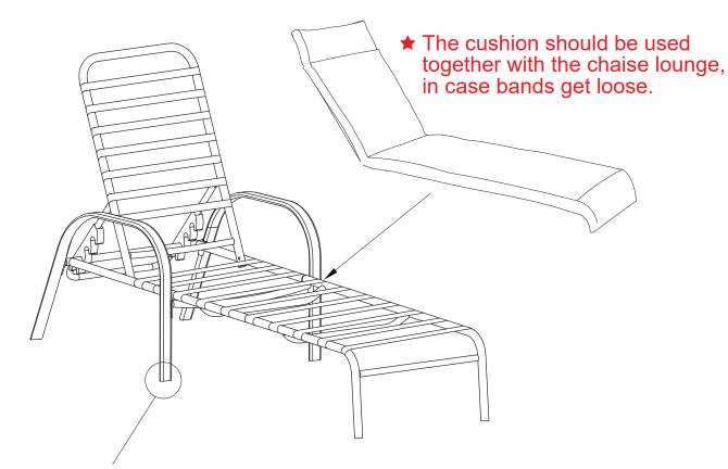
★ The middle leg is designed to not touching ground when assembled.
