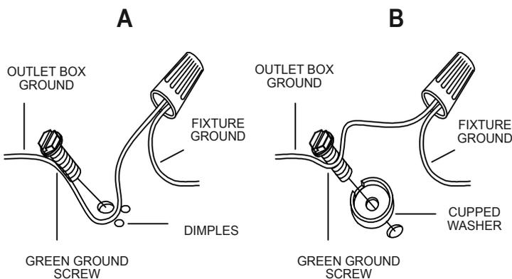
Connect wires according to the chart below
