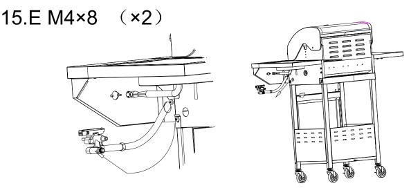
Step 1. Take out side burner gas valve from bottom of control panel
