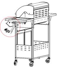
Step 1. Take out side burner gas valve from bottom of control panel
