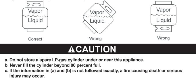
**NOTE:** Other cylinders may be acceptable for use with this appliance If they are compatible with the appliance nesting hole and retention means. Refer to Page11 of the Assembly Instructions for correct cylinder to cylinder holder connection.
