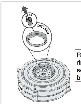
Remove the **ORANGE** shipping ring from the motor. **Save the screws. They will be needed for blade iron installation.**
