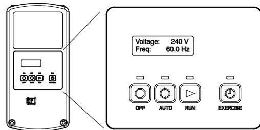
The DC2 controller provides integrated control for the generator set, Kohler® Model RXT transfer switch, programmable interface module (PIM), and load control module (LCM).
