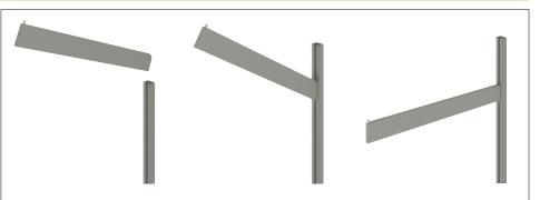
The bracket will be inserted into your WAL Standards on the smooth channel side while turned at a 45 degree angle. Insert the bracket through the top pr bottom of your WAL Standards. Carefully slide your bracket along the WAL Standards to the desired position. Begin to gently push the bracket down to snap into place.
