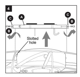
5. Secure mounting plate (A) to outlet box using screws, spring washers and flat washers provided with the outlet box.
