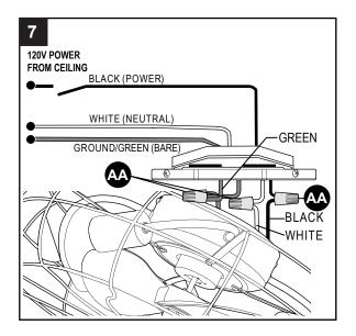
8. Wrap electrical tape (not included) around each individual wire connector (AA) down to the wire.
