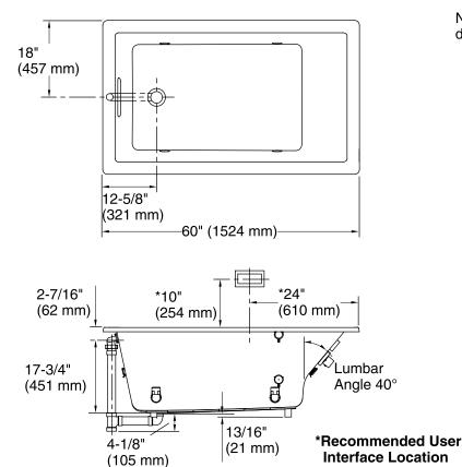
No change in measurement if connected with drain illustrated. (K-7272)
