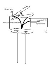
6 » Secure single bar (C) to the outlet box with mounting screws (B).
