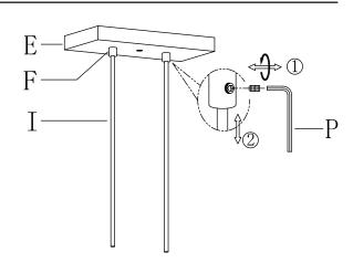
5 » If needed, shorten the extra length of the fixture wires from cords (I) so that they all are at least 6 inches (152.4 mm) long above canopy (E) within the outlet box.
