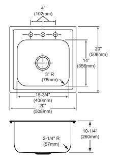
Hole Drilling Configurations
