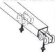
Place hangers in track by fitting through hanger mounting space between track and jamb.
