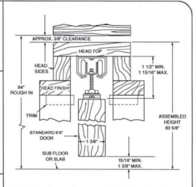
NOTE: Floor clearance is for a standard 80" door. Trim door accordingly for clearance over heavy carpet, etc.
