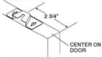
Screw all hanger brackets on door, 2 3/4" from edge of door to center of bracket.
