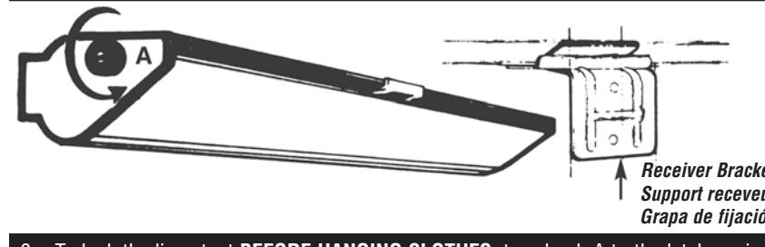
6. To lock the lines taut **BEFORE HANGING CLOTHES**, turn knob A to the latch position (clockwise) and then turn knob B (clockwise) to tighten the lines as desired. This procedure locks and tightens the lines so they are ready for use.
