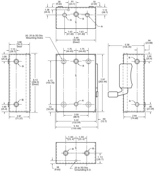
Dimensions shown in inches and millimeters ( ). Dimension shown accurate to  $\pm\,1\%$  inch. Note: Handle shown on front and right hand views only.
