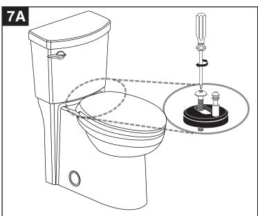
Put screws into seat hinge and tighten using a screwdriver.
