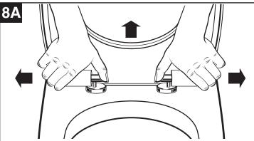
Open the seat and cover. Push both inside buttons to release seat and cover. Pull the seat and cover upwards to take it off the hinges.
