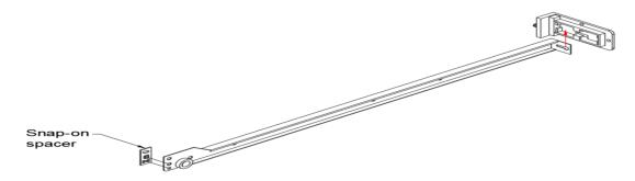
Make sure the slide is oriented as shown in detail below and snap 1/8" thick roll tray spacer onto cabinet member.
