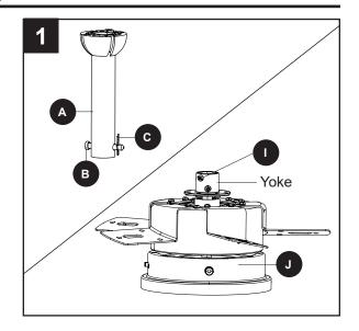
2. Insert the downrod (A) -- or a longer downrod (not included), if required -- through the canopy (E) and yoke cover (H). Feed the wires from the fan through the downrod (A).
