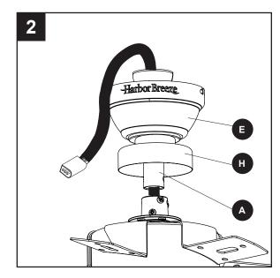
Slide the downrod (A) into the yoke, align the holes, then re-install the downrod pin (B) and downrod clip (C). Secure with set screws (I) and slide the yoke cover (H) down until it rests on top of the motor assembly (J).
