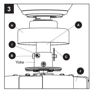
4. Depending on the length of downrod (A) you use, you may need to use the 36-inch lead wire (S) to accomodate a 36 or 48-inch downrod (sold separately). When necessary, connect the 3-pin connector extending from the center of the downrod (A) to one end of the 36-inch lead wire (S). Note: The downrod (A) included with this fan will not utilize the 36-inch lead wire (S).
