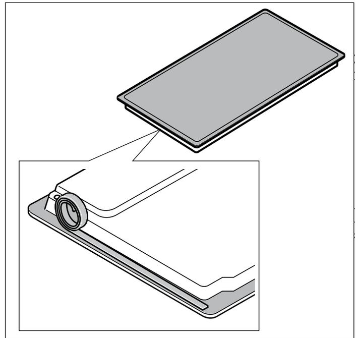
2. Screw each one of the clips into the position shown in the following image, so that they are free to rotate.
