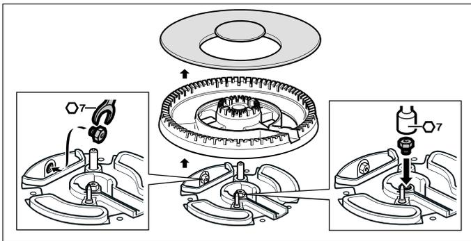
3. Fasten the nozzles and attach the burner caps to the corresponding burners. Put the burner grates in place on the corresponding burners.
