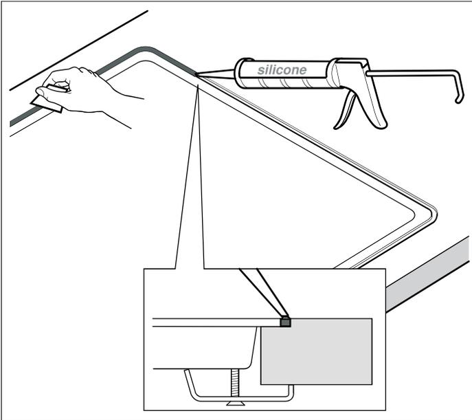
5. Allow the silicone sealant to dry before using the appliance.
