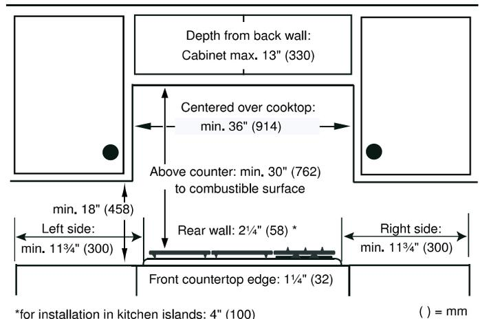
For installation in a kitchen island, the minimum distance from the cooktop to the edge of the countertop must be at least 4" (100 mm).
