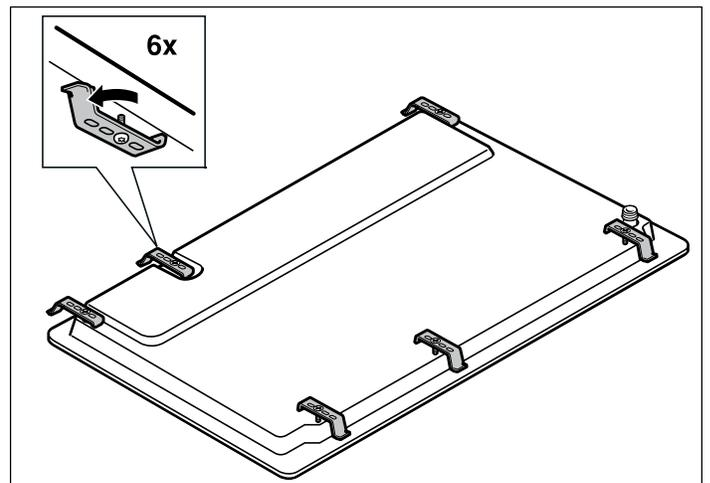
3. Turn the mounting brackets and tighten them fully. The orientation of the mounting brackets depends on how thick the countertop surface is.
