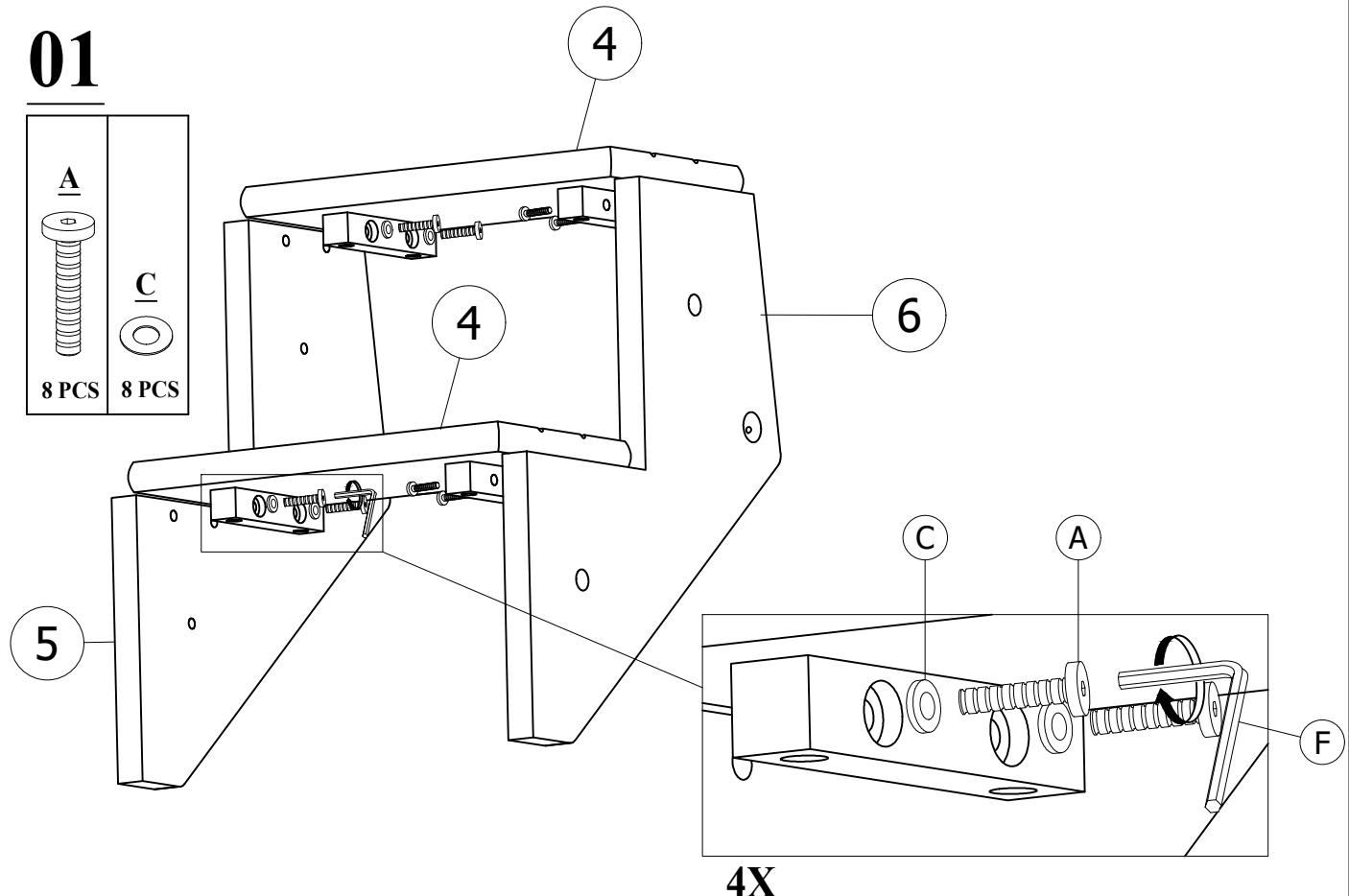
DO NOT TIGHTEN BOLT COMPLETELY UNTIL STEP 2 IS COMPLETE.
