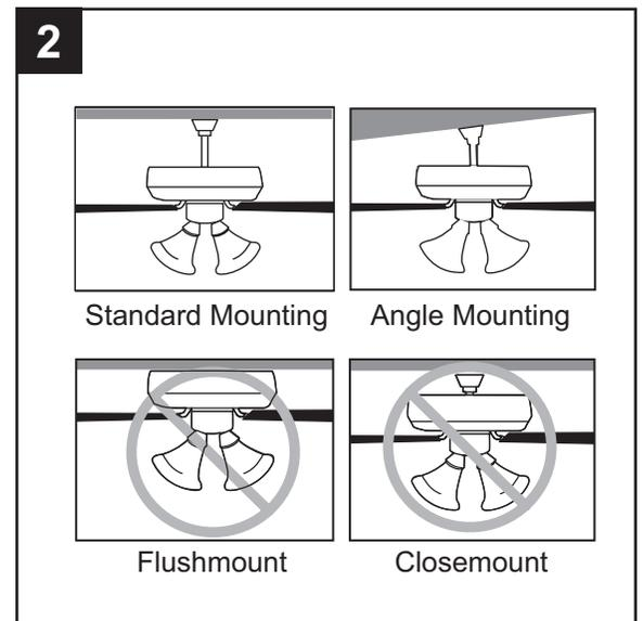
3. Ensure the blades (K) will be at least 30 in. from any obstructions. Also check the downrod (A) length to ensure the blades (K) will be at least 7 ft. above the floor.
