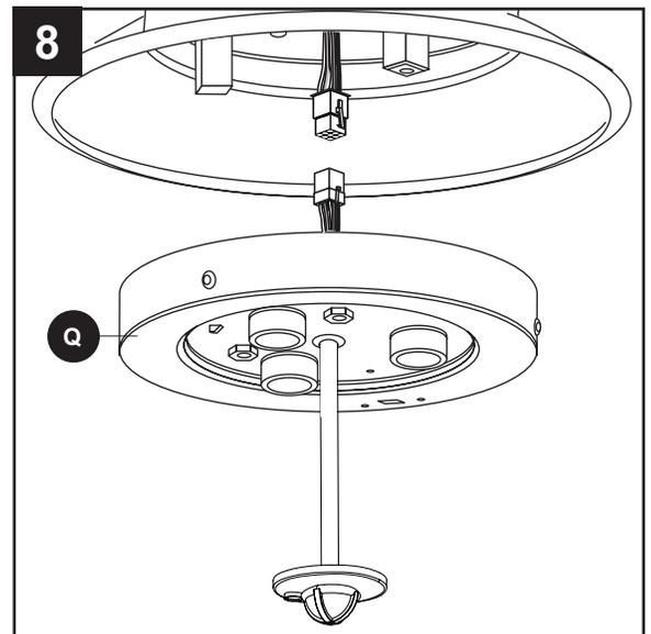
9. Align the two key slots in the light kit (Q) with the two previously loosened light pan screws (S). Place the light kit (Q) over the two screws and turn the light kit (Q) clockwise. Re-install the previously removed light pan screw (S) and tighten all three screws securely.
