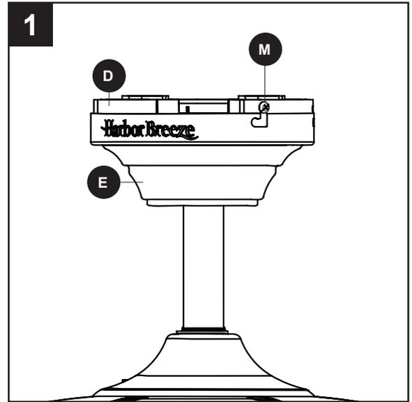
2. Secure the canopy (E) with the mounting bracket screws (M) previously removed (Step 4, page 8). Tighten all mounting bracket screws (M) securely.
