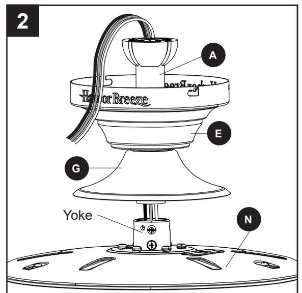
3. Slide the downrod (A) into the yoke of the motor assembly (N), align the holes, then re-install the downrod pin (B) and downrod clip (C). Secure with set screws (L).
