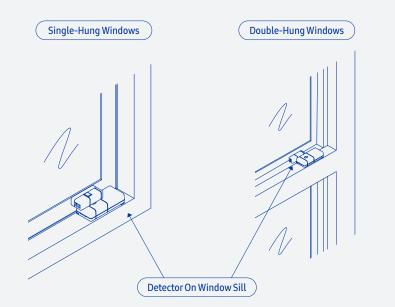
• Make sure that the alignment marks on both parts of the detector are aligned and facing each other, and that both parts of the detector are less than 0.5 inches apart when the door or window is closed
