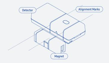
• Make sure the detector is placed at the top of door or window frames to avoid accidental damage to the detector.
