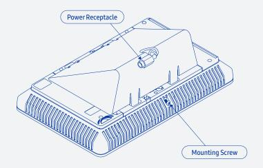
**3.** Connect the ADT Security Hub to a power outlet. Make sure the outlet is not controlled by a switch that could accidentally cut the power.
