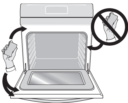
Figure 19: Clean around the oven door gasket
