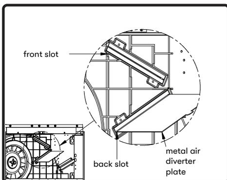
1. Remove the baffle filters. Remove air diverter plate slot covers. Remove metal air diverter plate from front slot and re-position to back slot. Re-install air diverter plate covers.
