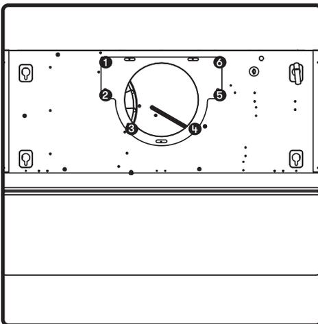
2. Secure 7" round collar to top of hood using (6) M4 x 6 screws.
