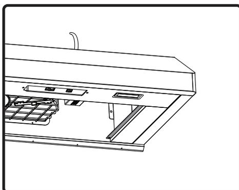
3. Remove all black foam from the filter opening before installing the charcoal filter brackets.
