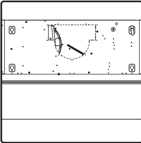
1. Using a flat-head screwdriver, remove both the rectangular and round knock-out plates located on top of hood.
