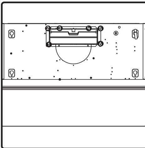
2. Secure 3-1/4" x 10" rectangular collar to top of hood using (6) M4 x 6 screws.
