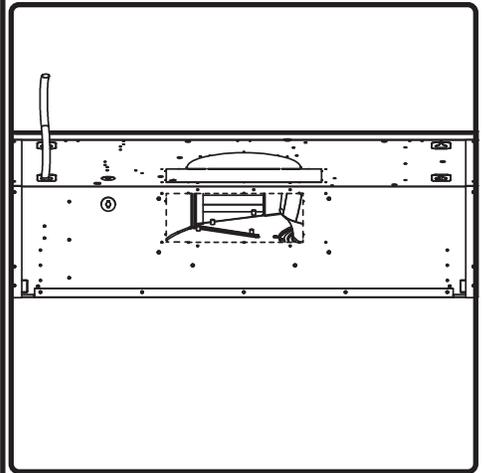
1. Using a flat-head screwdriver, remove the rectangular knock-out plate located on back of hood.
