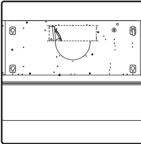
1. Using a flat-head screwdriver, remove only the rectangular section of the knock-out plate located on top of hood.
