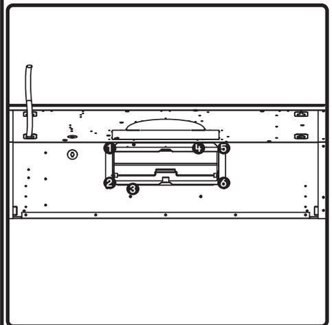
2. Secure 3-1/4" x 10" rectangular collar to back of hood using (6) M4 x 6 screws.
