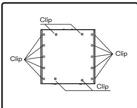
2. Using components from ZRC-0071, place (2) charcoal filter on the back of the baffle filters. Secure charcoal filters in place with rubber clips.
