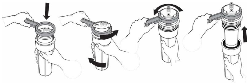
**STEP 3 Attach Cartridges**
