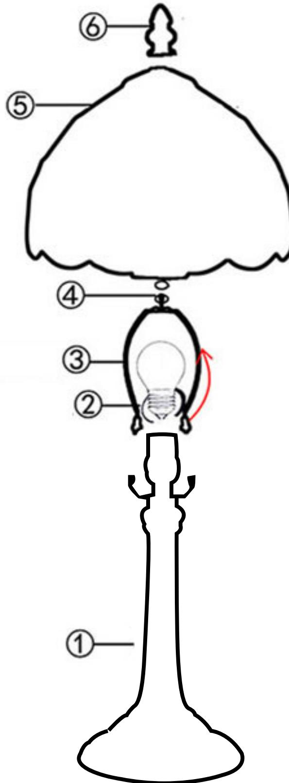
Install the light bulb, lift the small cover on the bracket, clip the bracket onto the base, place the lampshade on the bracket (gasket), screw on the cover, and secure the lampshade.
