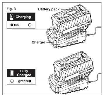
**4.** When the charger light turns green, the battery is fully charged (Fig. 3).
