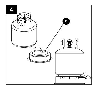
5. To install the propane gas tank to the body (B), first turn the cylinder valve on the propane gas tank clockwise to close the gas supply on the propane gas tank. Then, screw the regulator coupling from inside the body (B) onto the valve clockwise by hand only. Make sure it is fastened securely.
