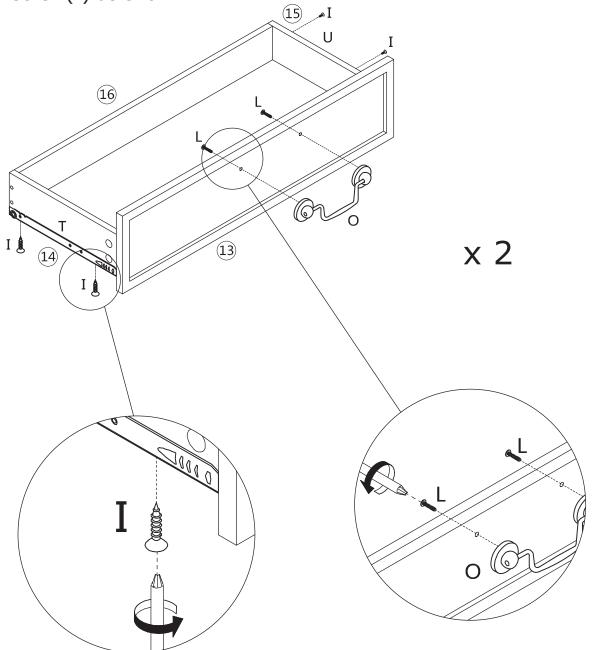
Fix handle(O) to plate 13 with screw(L) as shown.
