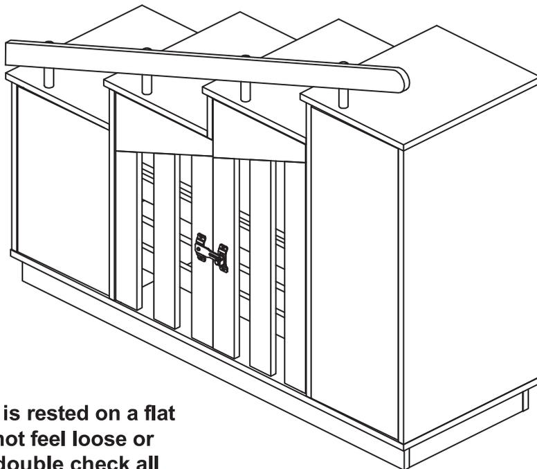
Make sure the unit is rested on a flat surface and does not feel loose or wobbly. If it does, double check all bolts/screws are secured and properly tightened.
