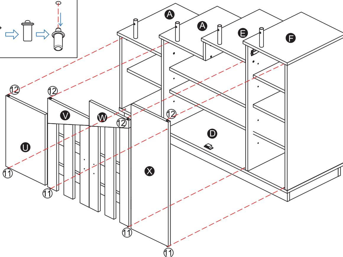
Insert non-spring assisted pin (#11) into the hole of the unit first before the spring assisted pin (#12).
