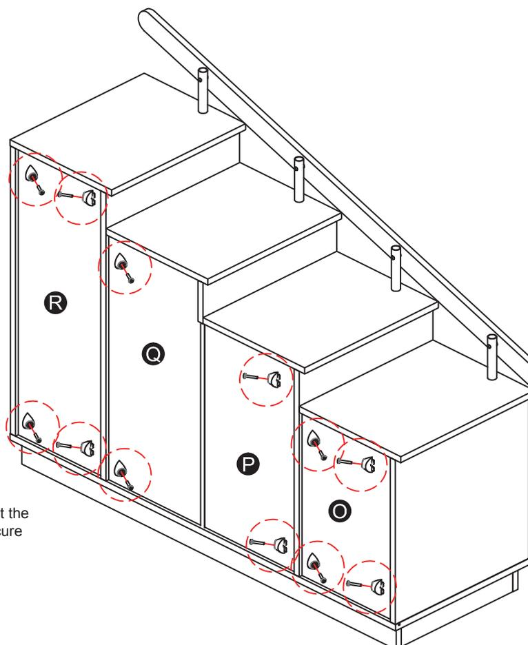
Insert fixative plates (#10) throughout the grooves of the back panels, then secure by using screws (#9).
