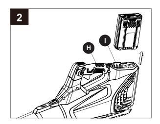
**Note:** The battery fits into the handle snugly in order to prevent accidental dislodging. It may require a strong pull to remove it.
