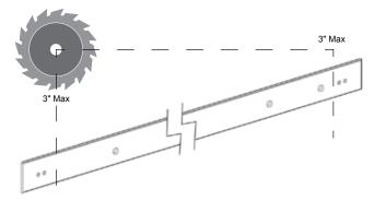
The rail can be trimmed if necessary using a band saw. Use blades suitable for iron or stainless steel depending on your rail.
