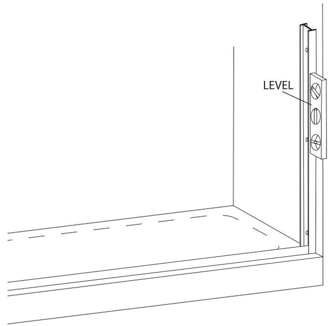
**3** Before replacing the tub track [A], force a slight downward bow in the extrusion. This will ensure the track fits tight to the tub. Run two beads of caulk inside the penciled marks on the tub rim. Place the tub track in the exact position marked in Step #2 and seat it firmly in the caulking.
