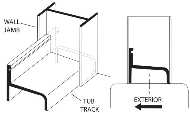
**2** Use a level to plumb both wall jambs [B], then mark the pre-drilled hole locations on the wall. Lightly mark along both sides of the tub track [A] with a pencil, then remove all parts.
