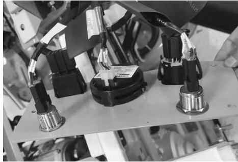
Connectors of the right operation enclosure
