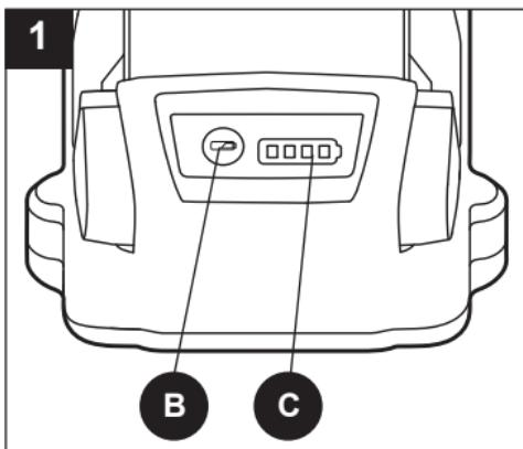
**NOTICE:** The power indicator can be used whether the battery is attached or removed from tool.
